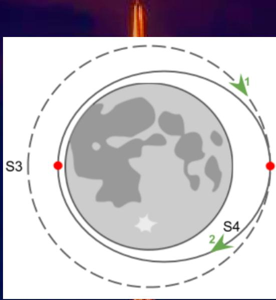
This process of getting closer to the moon usually takes a couple of days, and is necessary because landing onto the surface straight away would not only take too much fuel (due to the drastic change in trajectory) but would also cause the spacecraft to land too quickly, making it extremely difficult to control its landing speed.
